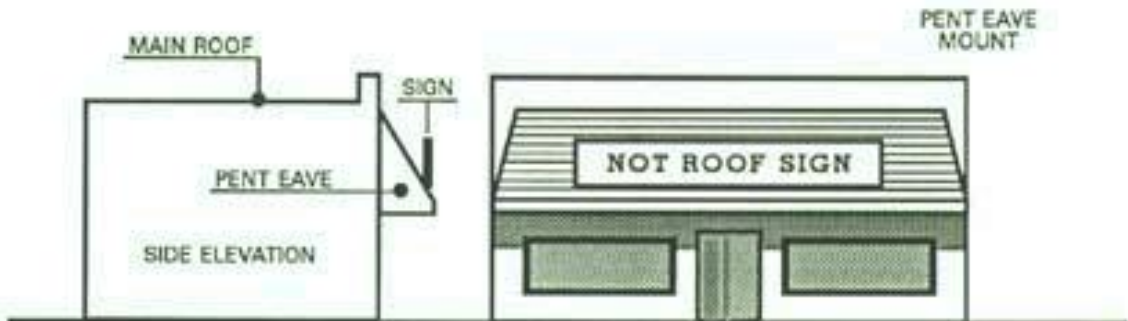
Figure 1003.2 Comparison - Roof and Wall or Fascia Signs
